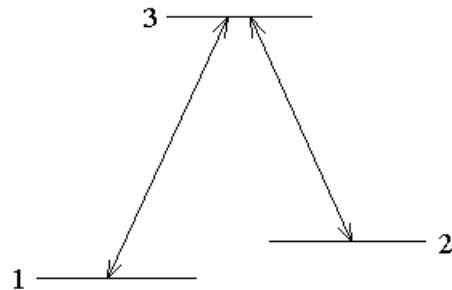
$$\left. \begin{array}{l} \omega - kV_z = \omega_{31} \\ \omega + kV_z = \omega_{32} \end{array} \right\} \Rightarrow \omega = \frac{\omega_{31} + \omega_{32}}{2} \quad \text{— условие формирования}$$
