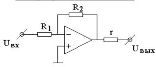
$$K_U \equiv \frac{U_{\text{BblX}}}{U_{\text{ex}}} = -\frac{R_2}{R_1}$$
