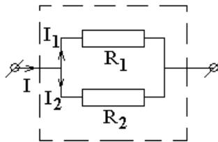
$$\begin{cases} U = U_1 = U_2 \\ I = I_1 + I_2 \end{cases} \Rightarrow \frac{1}{R} = \frac{I}{U} = \frac{I_1 + I_2}{U} = \frac{I_1}{U} + \frac{I_2}{U} = \frac{1}{R_1} + \frac{1}{R_2} \Rightarrow \frac{1}{R} = \frac{1}{R_1} + \frac{1}{R_2}$$
