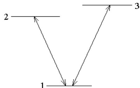
$$\left. \begin{array}{l} \omega - kV_z = \omega_{21} \\ \omega + kV_z = \omega_{31} \end{array} \right\} \Rightarrow \omega = \frac{\omega_{21} + \omega_{31}}{2} \quad — \text{условие формирования}$$
